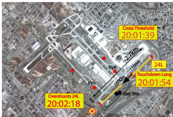
Figure 1: Image showing the runway orientation of the Lester B. Pearson Airport (YYZ) and the critical times as the plane approached from the upper right of the figure.
