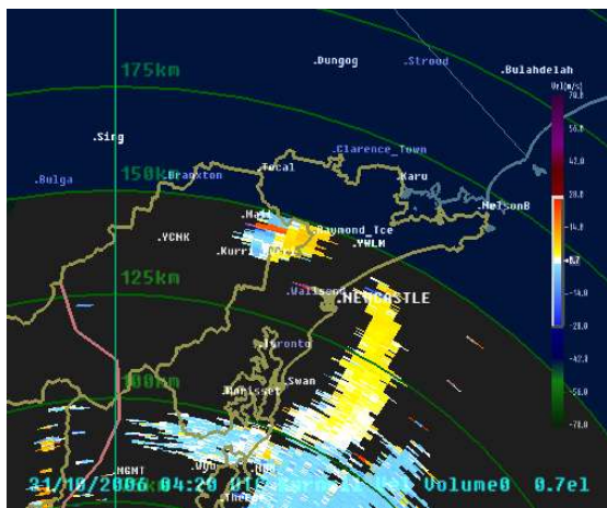
Figure 6. Velocity data for Kurnell radar on a 0.7-degree elevation angle PPI at 0420Z on 31 October 2006. Outbound winds are shaded orange and red, inbound winds in blue. The storm of interest is nearly 150 km distant from Kurnell radar and the PPI at this distance is about 3100 metres above ground level.
