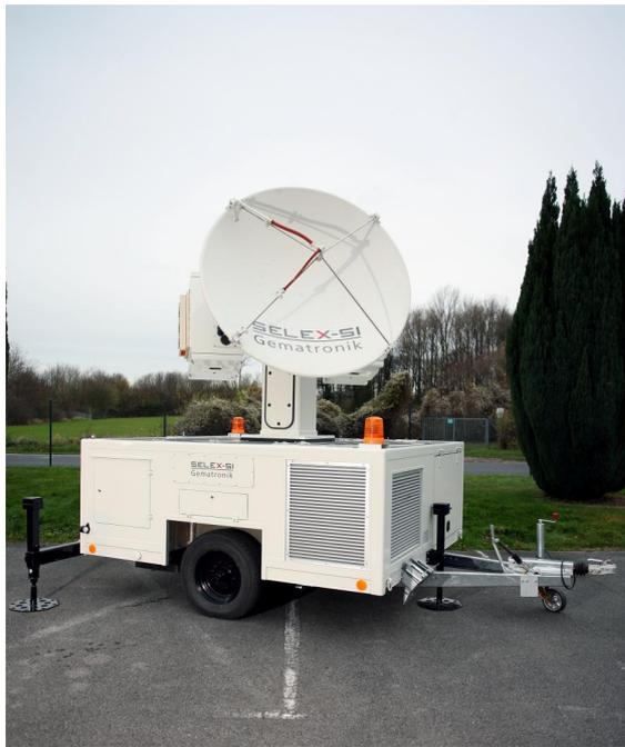
**Figure 4:** Trailer radar without radome installed. For standard setup the trailer is mounted on support feeds. The alignment for operation is done by mechanical leveling (0.05°), built in GPS and solar calibration.
