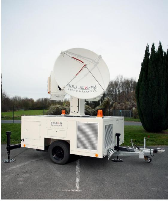
**Figure 4:** Trailer radar without radome installed. For standard setup the trailer is mounted on support feeds. The alignment for operation is done by mechanical leveling ( $0.05^\circ$ ), built in GPS and solar calibration.
