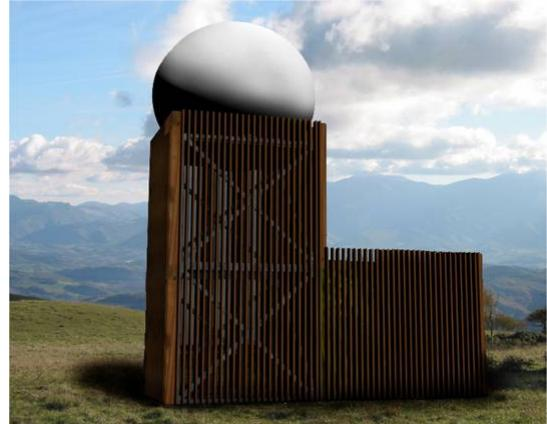
**Figure 3:** Sketch of a typical fixed installation. The radar can be installed on top of a roof as well, with and without radome protection.
