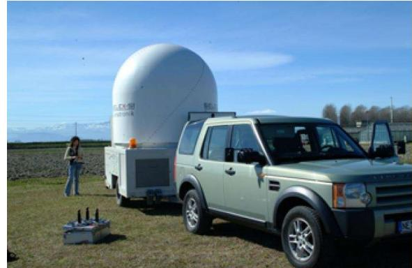
**Figure 1:** Mobile trailer radar attached to the towing vehicle. The weight of the trailer is 2.8 tons including radome.
