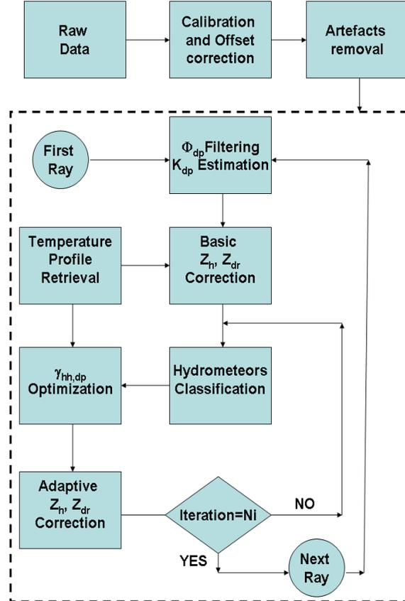
Figure 1. Block diagram of the proposed attenuation correction scheme with embedded hydrometeors classification.
