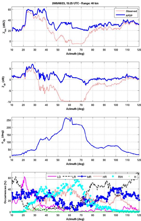
Figure 4. Plot of observed and corrected  $Z_{nh}$  (upper panel) and  $Z_{dr}$  (middle panel) as a function of the azimuth (between 10 and 120 degrees) for a fixed range distance (40 km) relatively to the event of June 23<sup>rd</sup> 2005 at 15:25 UTC. The third and fourth panels show the corresponding plots of  $\phi_{dp}$  and identified hydrometeor classes (i.e, Large Drops LD, Light Rain LR, Moderate rain MR, Heavy Rain HR, Rain/Hail R/H, Hail H), respectively.
