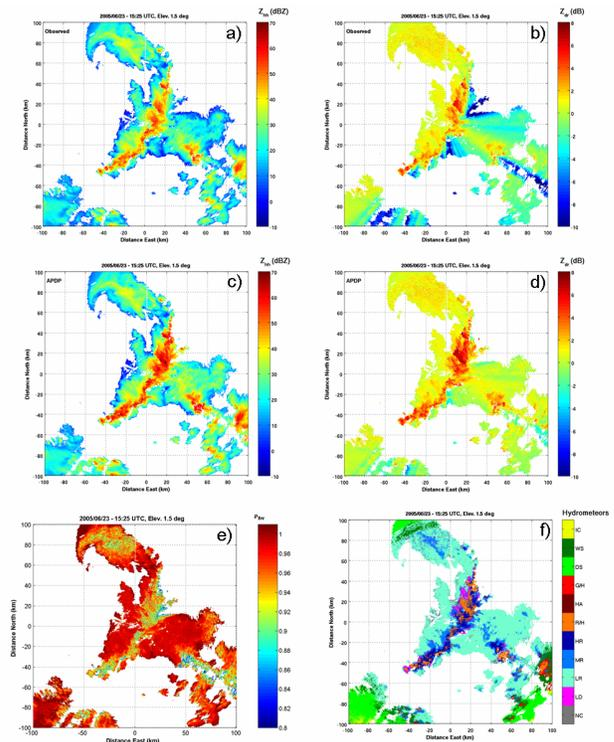
Figure 3. PPIs of polarimetric radar variables and the corresponding hydrometeor types (Fig. 3 f). Figures 3 a-d) show the observed (a,b) and corrected (c,d)  $Z_{hh}$ ,  $Z_{dr}$ , respectively. Figure 3 e) shows the correlation coefficient.
