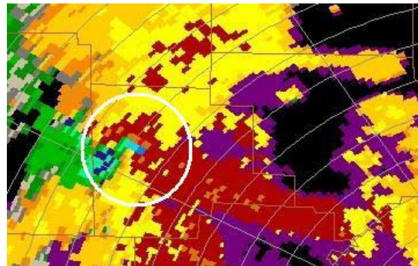
Figure 8. 2102 UTC 0.5 deg storm-relative velocity (BMX) showing gate-to-gate maximized (magnitude > 50 \text{ kt} , > 25 \text{ m s}^{-1} ) inbound and outbound velocities.
