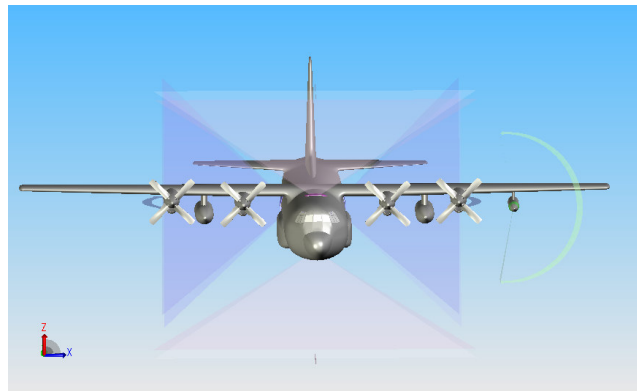
Figure 3: C-130 Front view showing beam envelopes of all four AESAs
