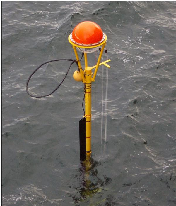
**Figure 3.** The NOC spar buoy. Wave wires are located on the right of the image. The underside of the dome is transparent and contains still and video cameras to image the region around the wave wires
