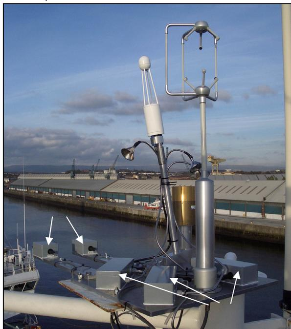
**Figure 1.** The flux installation on the foremast. The CLASP inlets are situated just below the LiCOR
