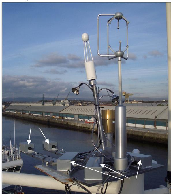
**Figure 1.** The flux installation on the foremast. The CLASP inlets are situated just below the LiCOR
