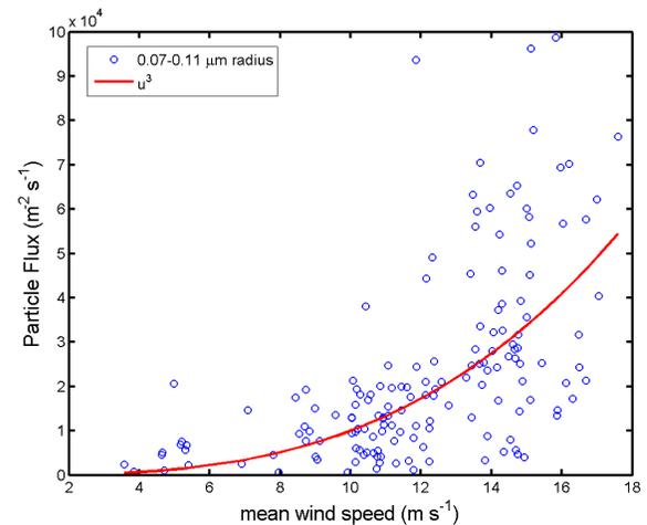
**Figure 4.** The sea spray flux data showing its cubic dependence on local wind speed.
