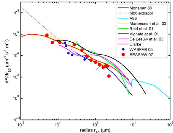
**Figure 5.** Comparison of preliminary flux estimates as a function of particle size for  $U_{10} = 5 \text{ m s}^{-1}$ , with those from a coastal site (WASFAB 06) and a number of recent parameterizations from the literature.
