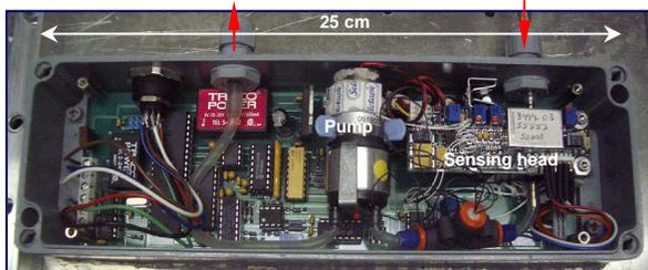
**Figure 2.** Internal layout of CLASP unit, red arrows indicate sample flow into the sensor head and exhaust from pump.
