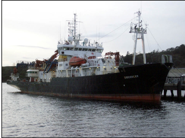
Figure 2. The RRS Discovery in port in Stornoway, showing the foremast with turbulence instrument installations.
