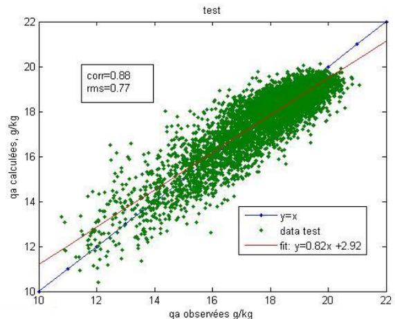
Fig.2 Comparison between retrieved qa by Neural Network and qa observed by buoys. AMSU
