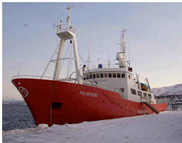
Figure 1. The Polarfront during a brief port call in Aalesund. The flux sensors are on the starboard side of the foremast platform.
