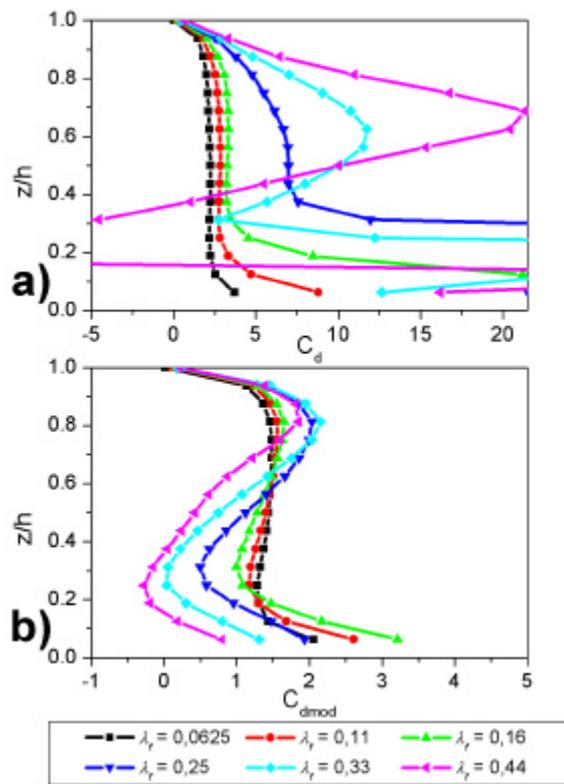
**Figure 3.** Vertical profiles of **a)**  $C_d(z)$  and **b)**  $C_{dmod}$  with packing density of the array of cubes calculated with RANS with  $k-\epsilon$ . Results are shown for  $I_f = 0.0625, 0.11, 0.16, 0.25, 0.33, 0.44$ . Note that the horizontal scales for  $C_d(z)$  and  $C_{dmod}$  are not the same.
