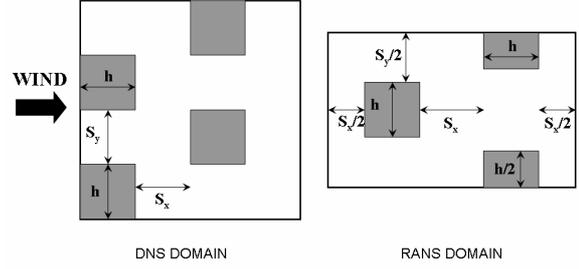
**Figure 1.** Plan view of the numerical domains corresponding to the DNS and RANS simulations.
