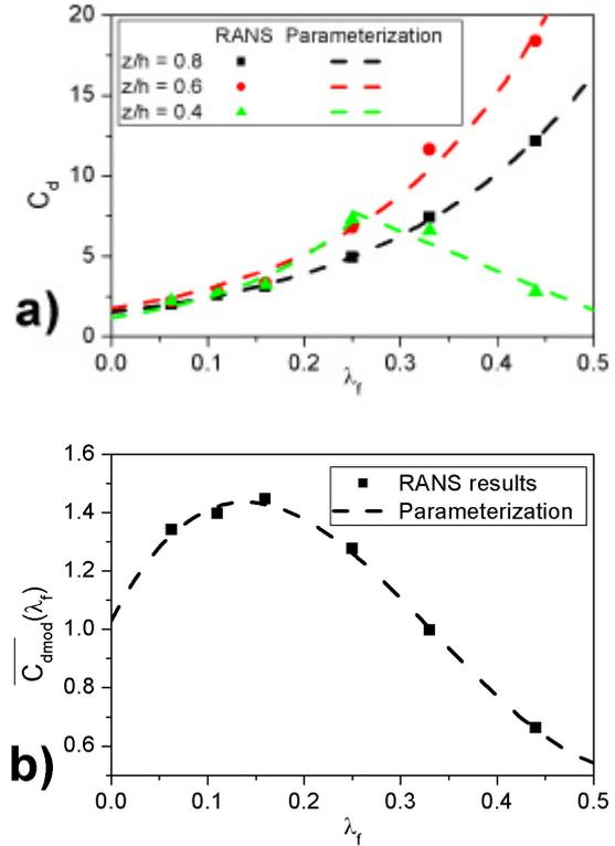
**Figure 4.** Variation of **a)**  $C_d(z/h, I_f)$  with  $I_f$  at  $z/h = 0.8, 0.6$  and  $0.4$  (dots are RANS model results and lines are the proposed parameterization) **b)**  $\bar{C}_{dmod}(I_f)$  with  $I_f$  (squares are RANS model results and dash line is the proposed parameterization).
