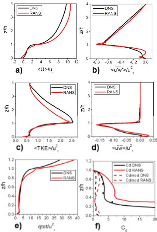
**Figure 2.** Comparison of vertical profiles of spatially-averaged statistics (a) mean streamwise wind speed, b) Reynolds shear stress, c) dispersive stress, d) turbulent kinetic energy, e)  $q_{tot} = \langle \overline{U} \rangle^2 + v_{TKE}^2 + v_{DKE}^2$  and f)  $C_d(z)$  and  $C_{dmod}$  from the DNS (solid line) and RANS simulations (dashed) in the case of  $I_f = 0.25$ . Values of  $C_d(z)$  computed from the experimental results of Cheng and Castro (2002) are also shown.
