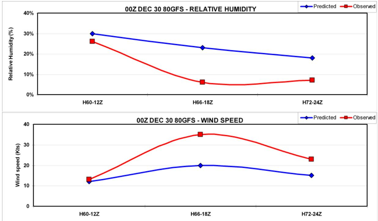
Figure 6: A graphical comparison of model-predicted 2 m relative humidity and 10 m wind speeds to observed values at KLBB using the 60 to 72 hour forecast from the 0000 UTC 30 December 2005 80GFS valid between 1200 UTC and 2400 UTC 1 January 2006. *Click image to return to main manuscript.*
