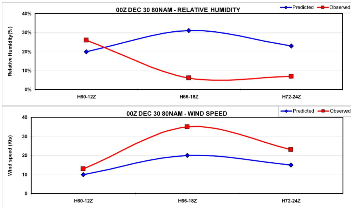
Figure 3: A graphical comparison of model-predicted 2 m relative humidity and 10 m wind speeds to observed values at KLBB using the 60 to 72 hour forecast from the 0000 UTC 30 December 2005 80NAM valid between 1200 UTC and 2400 UTC 1 January 2006. [Click image to return to main manuscript.](#)
