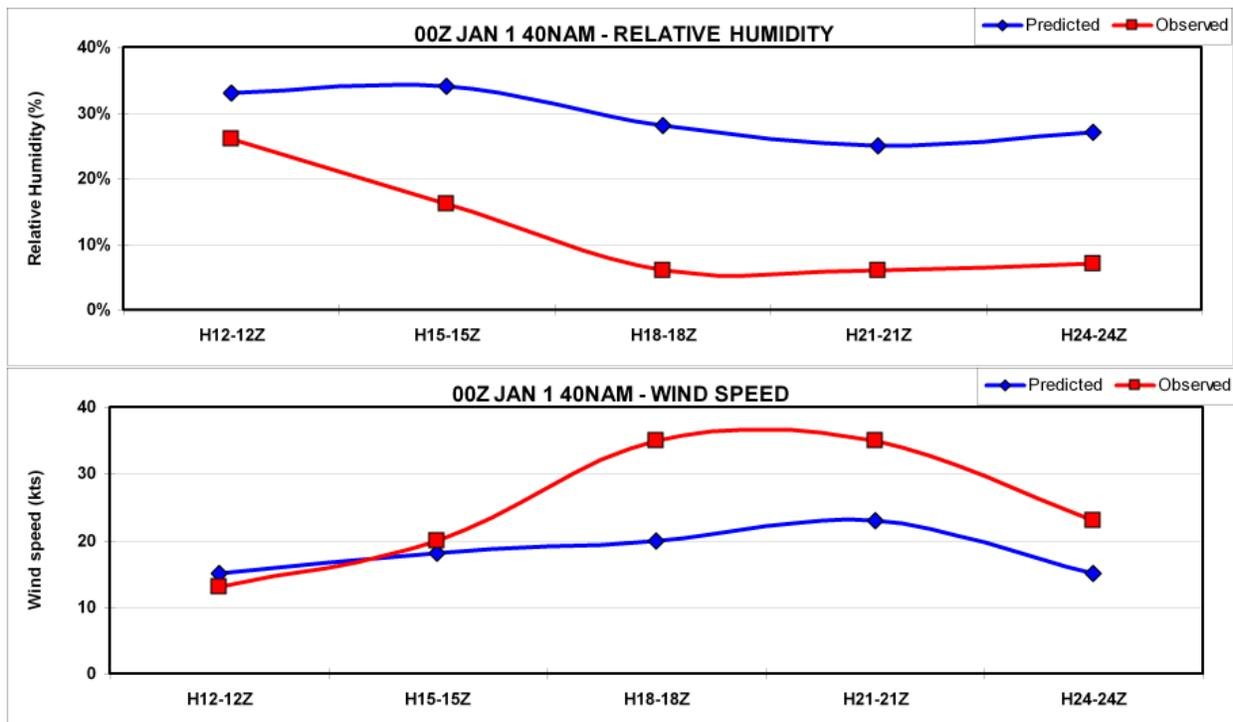
Figure 5: A graphical comparison of model-predicted 2 m relative humidity and 10 m wind speeds to observed values at KLBB using the 12 to 24 hour forecast from the 0000 UTC 1 January 2006 40NAM valid between 1200 UTC and 2400 UTC 1 January 2006. *Click image to return to main manuscript.*
