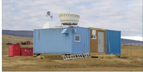
Figure 2: The MMCR and HSRL in their seatainer, near Eureka. The former is visible from its antenna on the top of the light blue seatainer, while the latter is recognized by its window, behind the MMCR antenna.
