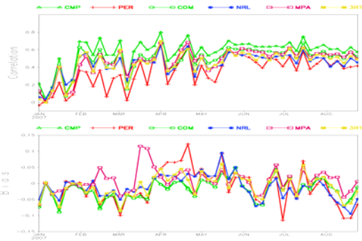
Fig.6 Time series of pattern correlation and bias between our gauge-based analysis and the selected satellite precipitation products on 0.25°lat/lon grid boxes and in 3-hourly time-resolution. Only data over grid boxes with at least one gauge are included in calculating the statistics.
