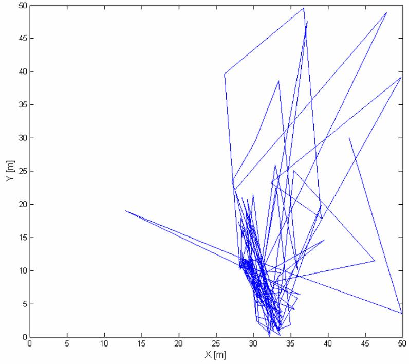
Figure 9. The simulated annealing search for the source location (every thousandth step).
