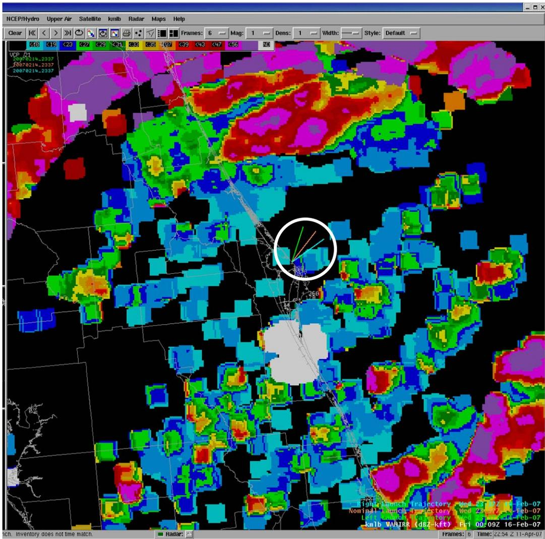
Figure 3. An example of the automated VAHIRR product as viewed in AWIPS. The Archive level II data is not the same as that in Figure 1. A white circle has been drawn around a left, nominal, and right launch trajectory.
