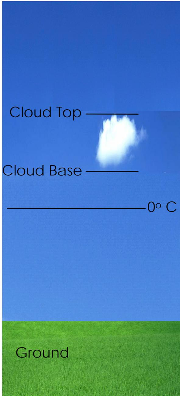
Figure 1. Depiction of the cloud top and base in VAHIRR. To take into effect vertical grid spacing, half a vertical grid spacing is then added to the cloud top and subtracted from the cloud base.
