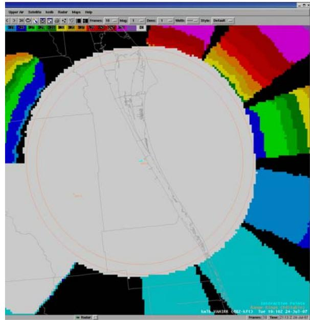
Figure 16. VAHIRR product in AWIPS with a cone of silence height of 58.62 kft (17.867 km). The inner range ring shows the calculated horizontal extent of the cone of silence. The radius of the outer range ring is 5 km larger than that of the inner range ring.
