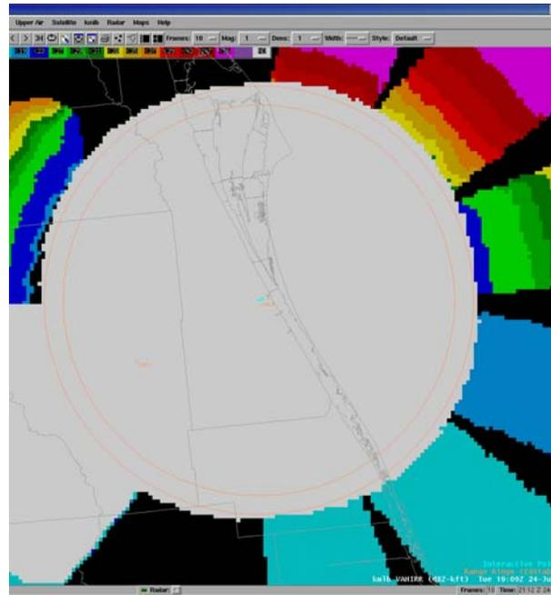
Figure 15. VAHIRR product in AWIPS with a cone of silence height of 59.74 kft (18.209 km). The inner range ring shows the calculated horizontal extent of the cone of silence. Invalid grid points are displayed in light gray. The radius of the outer range ring is 5 km larger than that of the inner range ring.
