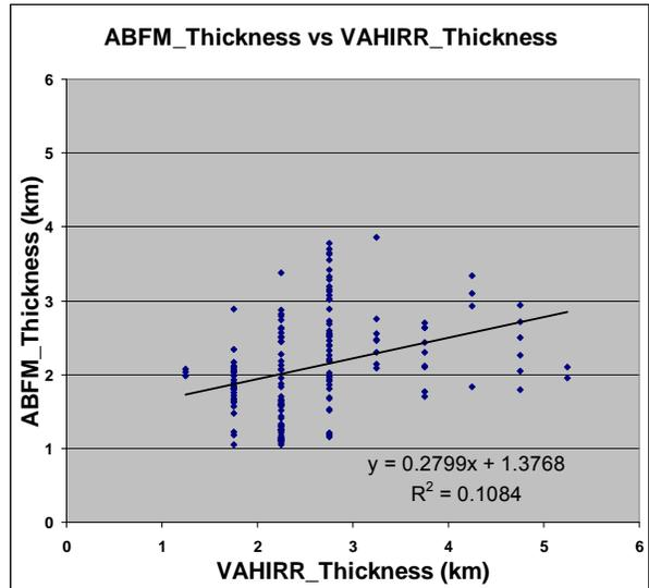
Figure 20. From the ABFM comparison test procedure, the average cloud thickness in the Volume Integral product versus the VAHIRR product.
