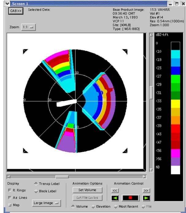
Figure 5. The VAHIRR product in the Initial Test, using the customized radar data.
