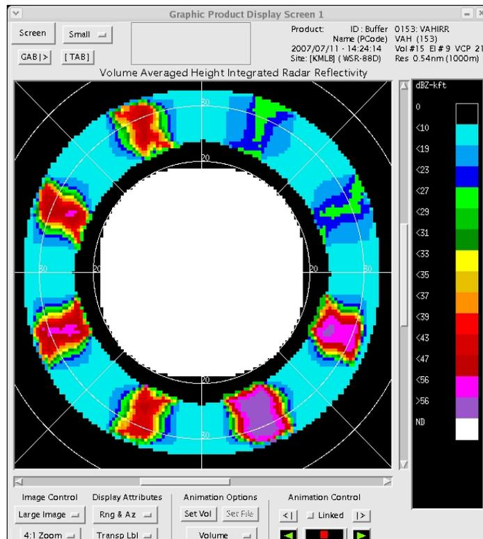
Figure 18. VAHIRR product in the Reflectivity Average for Multiple Tilts Test procedure.
