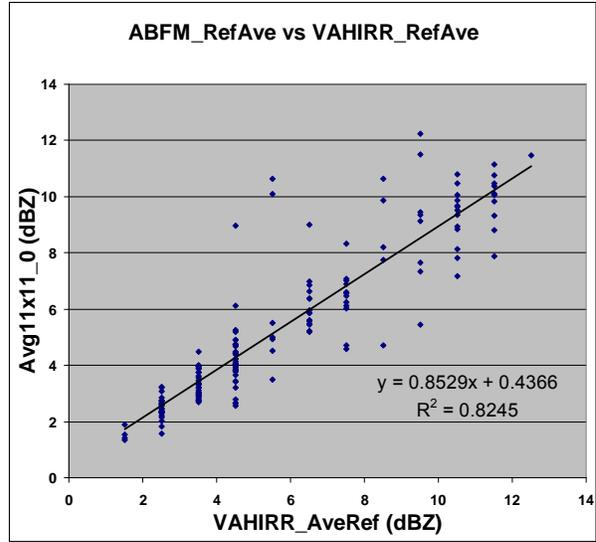
Figure 19. From the ABFM comparison test procedure, the volume averaged reflectivity in the Volume Integral product versus the VAHIRR product.
