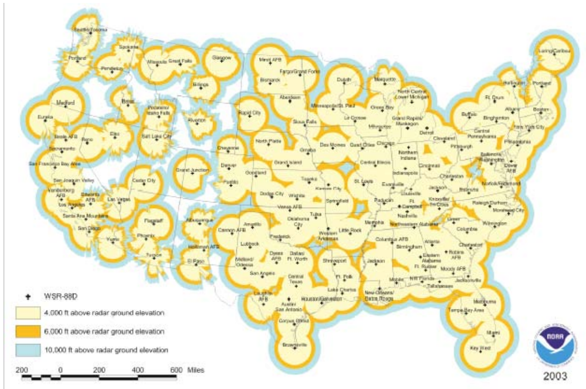
Doppler weather radar coverage of CONUS at 4,000, 6,000, and 10,000 feet above radar ground elevation from the nationwide network of WSR-88Ds (Next Generation Weather Radars). (Courtesy of SRI International)
