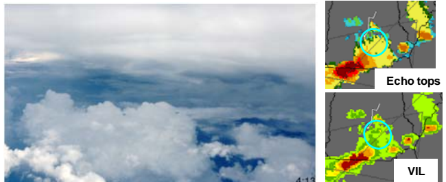
Figure 9. Photographs showing a thunderstorm anvil overhang (a), taken from 28 kft., and a region of high echo top decay behind the leading edge of a storm (b), taken from 35 kft. Pilots tend to avoid anvils, where convective activity is vigorous and growing and where flights will experience significant turbulence. Pilots are more likely to penetrate or fly over regions of high-topped decay, where convective activity is weak and turbulence is minimal.
