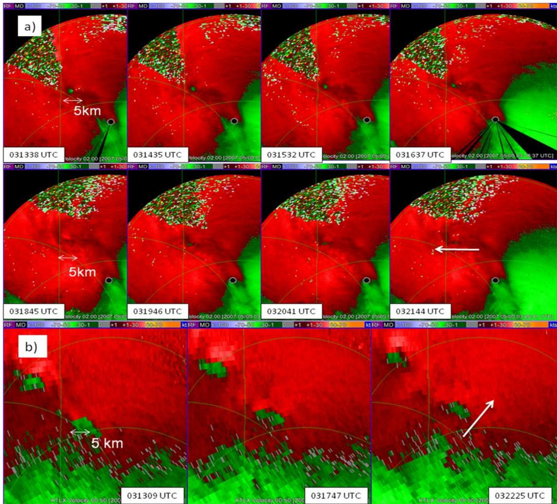
Figure 12: a) Velocity data collected from the CASA radar near Chickasha (KSAO) at 2 degrees elevation at times 031338, 031435, 03413, 031532, 031637, 031845, 031946, 032041 and 032144 UTC. b) Velocity data collected from the WSR-88D radar at Twin Lakes, OK (KTLX) at 0.5 degrees elevation at times 031309, 031747, and 032225 UTC.
