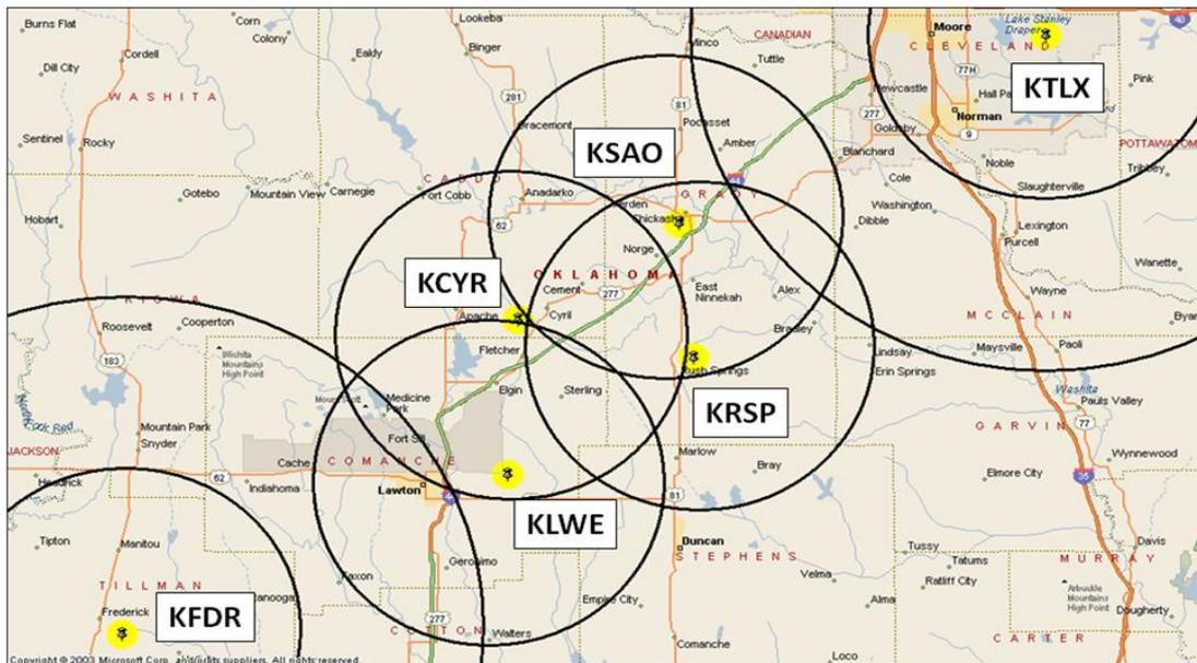
Figure 1: The first CASA testbed is located in southwestern Oklahoma. The four radars are located in or near the towns of Chickasha (KSAO), Cyril (KCYR), Lawton (KLWE), and Rush Springs (KRSP). The nearest WSR-88D radars are near the towns of Frederick (KFDR) and Twin Lakes (KTLX). Range rings of 30 km and 60 km are marked.
