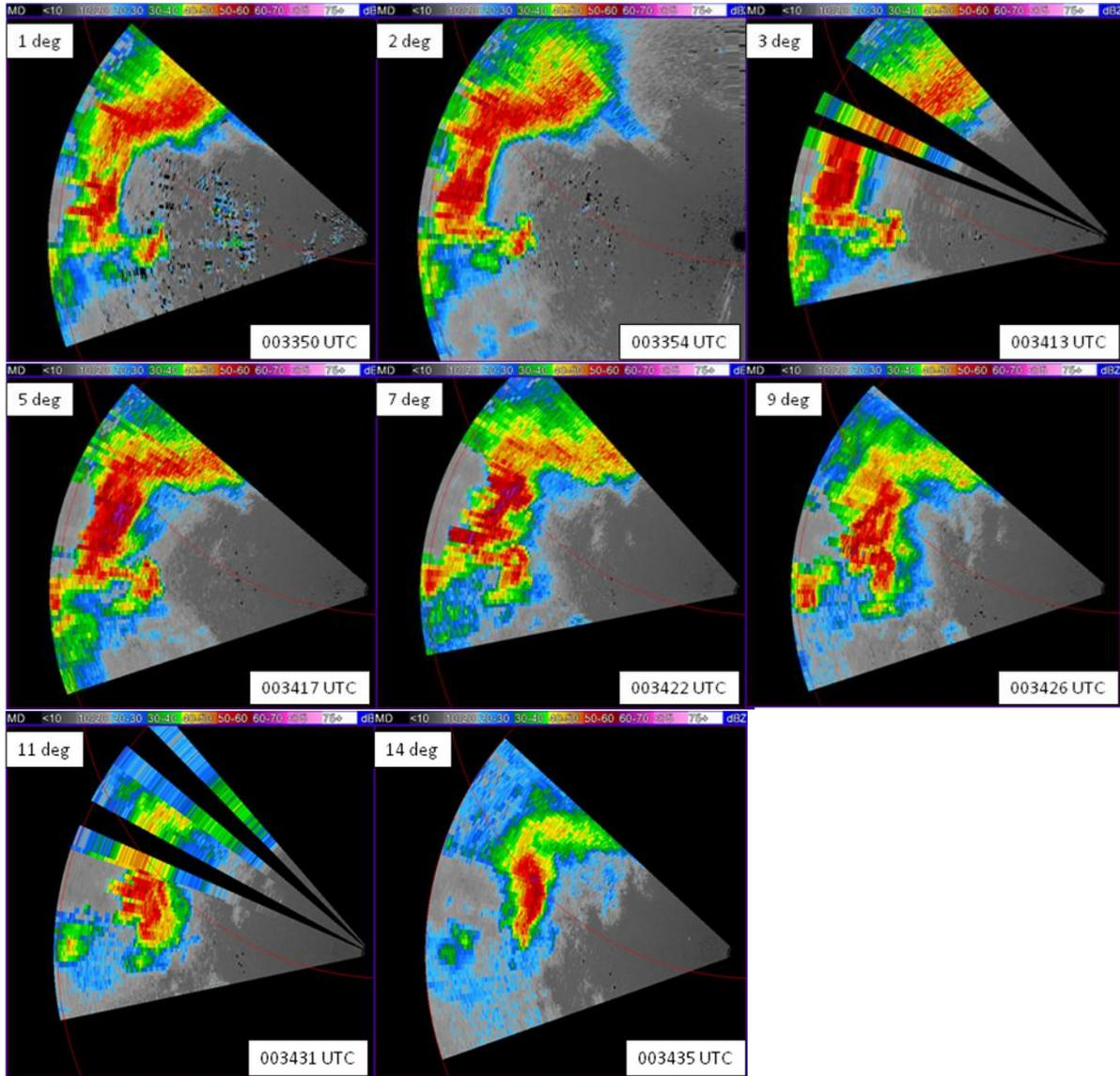
Figure 10: A demonstration of the adaptive, sector scanning capabilities. Reflectivity data collected at 1, 2, 3, 5, 7, 9, 11, and 14 degrees elevation at times 003350, 003354, 003413, 003417, 003422, 003426, 003431, and 003435 UTC, respectively.
