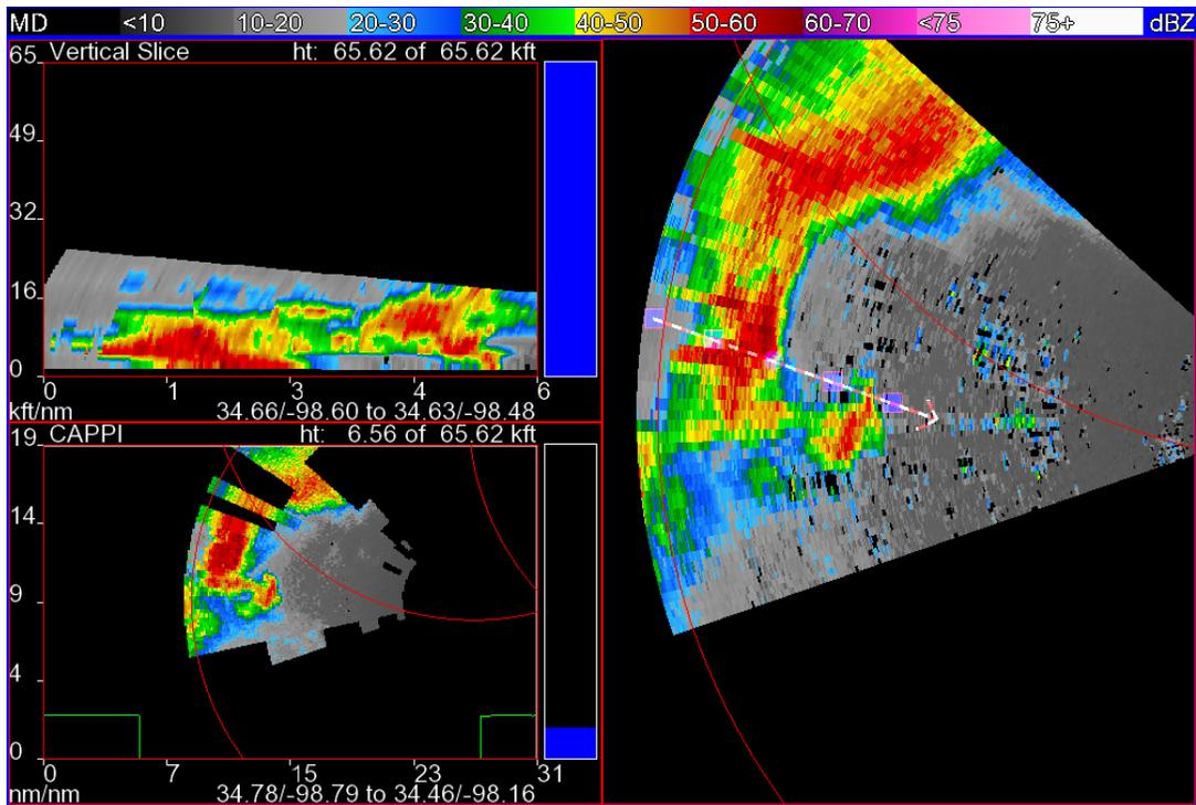
Figure 11: A vertical slice image created from the consecutive PPI slices. Because of the adaptive scanning capabilities, a full volume scan of the storm can be completed and displayed once per minute.
