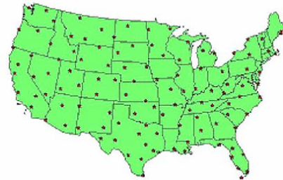
Figure 1: Today's NLDN consisting of 113 lightning sensors locations across the continental US (Grogin.)
