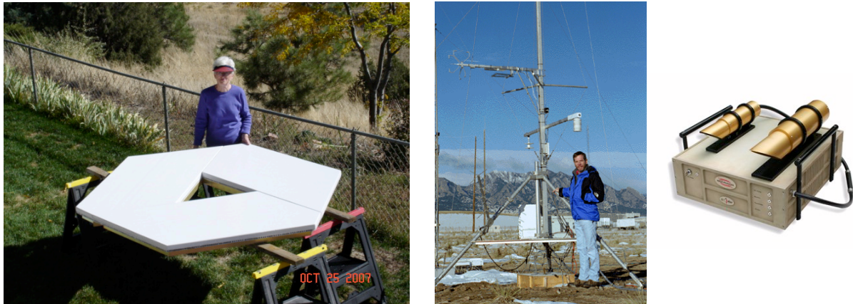
Figure 1: Three components of the MPN stations, a prototype antenna module for the wind profiler (left, photo by Warner Ecklund), a surface flux tower (center), and mini-Doppler lidar (right, HALO-Photonics).
