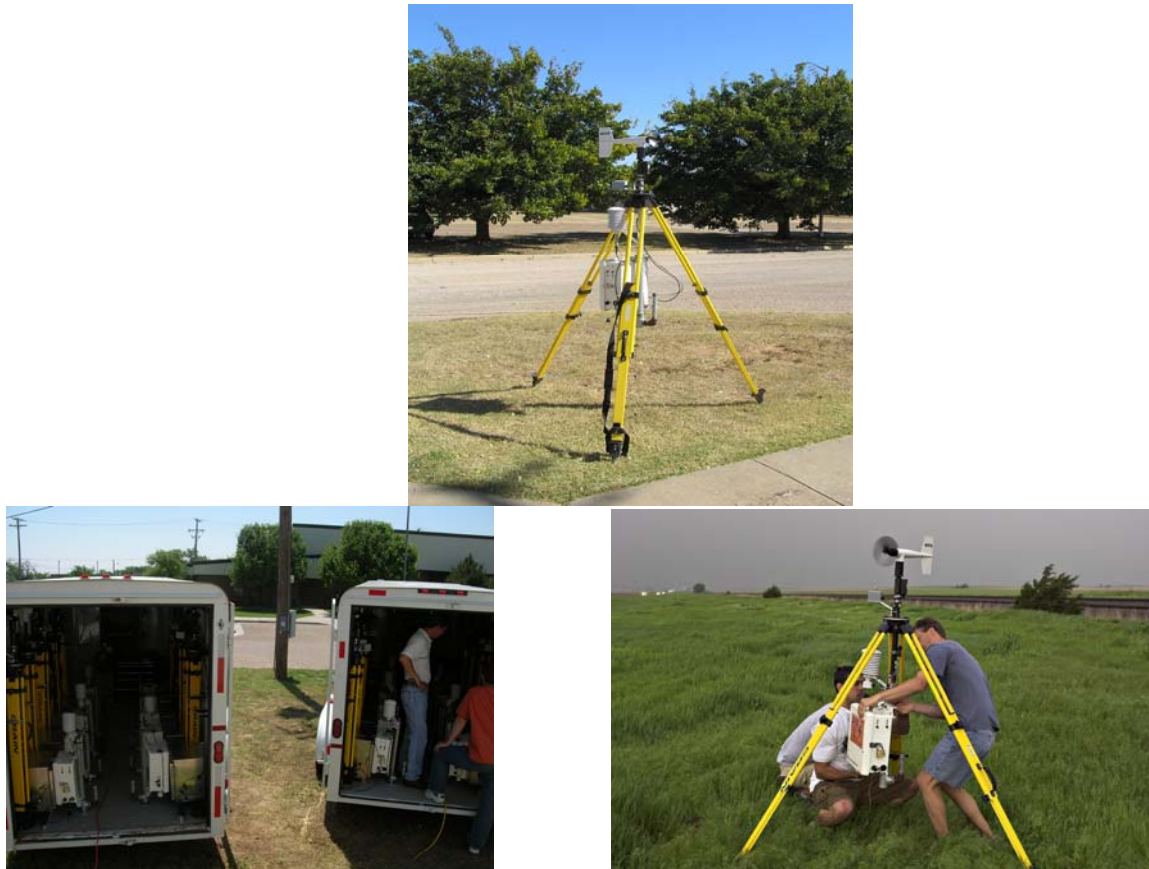
FIGURE 1 – Photographs of a StickNet station (top), transport trailers (lower left) and deployment (lower right) during the Spring 2007 field project.
