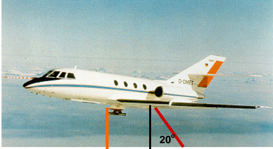
Figure 1: DLR Falcon employed during IHOP indicating nadir DIAL beam (orange) and Doppler beam (red), directed at 20 degree nadir angle transverse to the flight direction.
