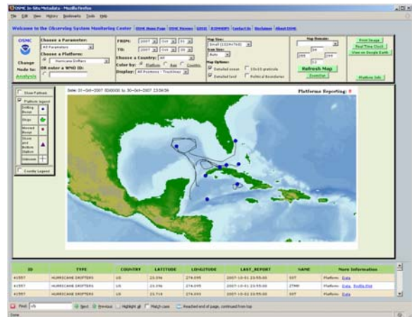
Figure 3. OSMC displaying Hurricane drifters, with track lines and metadata, for the month of October 2007
