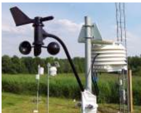
FIG. 1. Vantage Pro Temperature/Humidity Station with Anemometer
