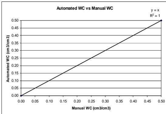
**Figure 3.** The ideal correlation between the Mesonet WC and the manually determined WC.
