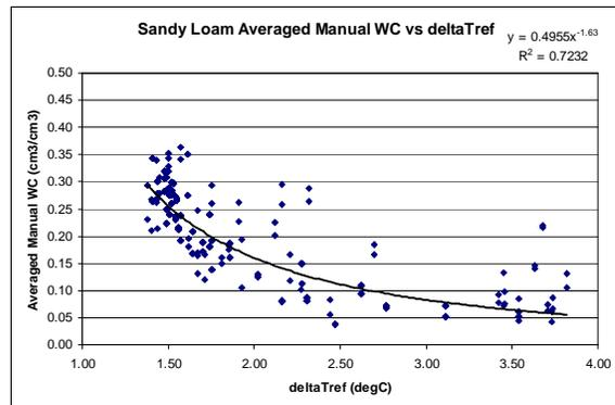
**Figure 8.** The relationship between the manual samples of WC and  $\Delta T_{ref}$  observed at Mesonet sites for sandy loam soils.
