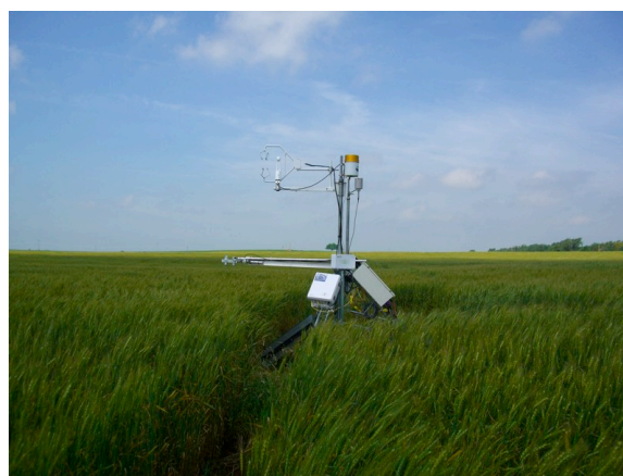
Figure 1 - Eddy covariance flux tower in a wheat field
