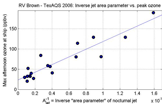
**Figure 4.** Ship-measured peak ozone versus the inverse of the nocturnal jet area parameter  $A_{\text{jet}}$ .
