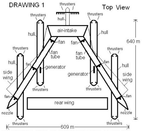
The machine is a ship, the ship has five torpedo shaped hulls. Each hull has rotating thrusters on it. The upper part of the ship is a V shaped turbo-charged wedge, each side of the V has three fan-tubes stacked vertically. Inside each fan-tube there are three high speed fans. The fans accelerate the air in the fan-tubes to 1900 km/h. There is a air-intake in the front of the machine and adjustable nozzles in the rear. There is a adjustable rear wing.
