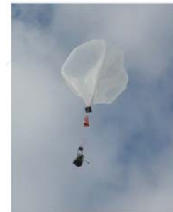
Fig. 4. Picture of a Driftsonde balloon with dropsonde gondola.
