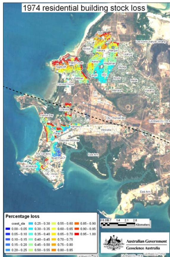
Figure 2: Estimated damage to residential building stock (1974 buildings) caused by TC Tracy.
