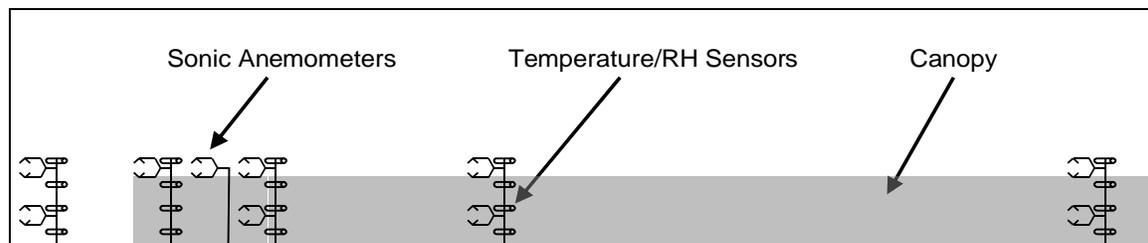
Figure 1, Diagram showing the location of the primary sensors used. The figure is not to scale. The mature canopy is 1.1 m tall, and the downwind measurements (at the right-hand side of the figure) are 144 m from the edge of the canopy.
