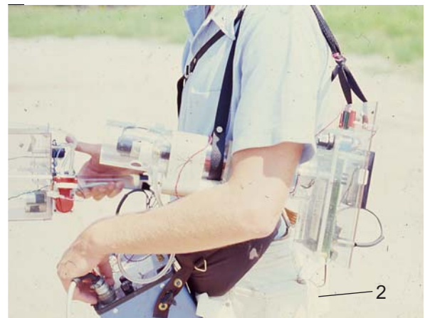
Figure 7: A field portable photosynthesis system in five pieces: 1) Liston-Edwards gas analyzer optical bench and board; 2) the analyzer power supply; 3) LI-1600 console; 4) Leaf chamber; 5) Tape recorder for data logging.
