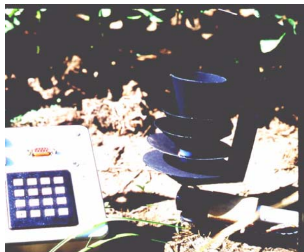
Figure 11: the Pine Cone Sensor shown with a Campbell Data Logger. When used in direct sun, it had a shadow band, shown on the right.
