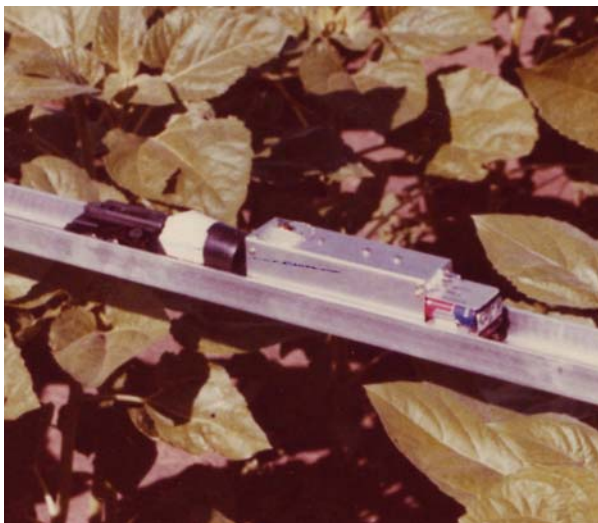
Figure 10: Sunflecks measured with a model train. The locomotive had to be "streamlined" a bit to prevent snagging foliage.
