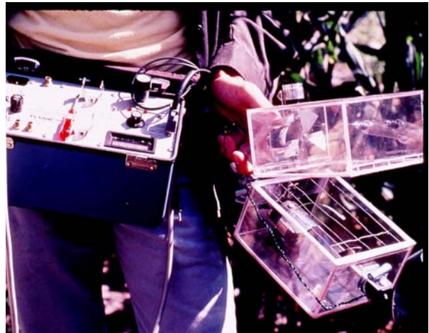
Figure 6: LI-1600 steady state porometer modified to measure humidity in a leaf chamber equipped with CO 2 syringes, barely visible on the right.
