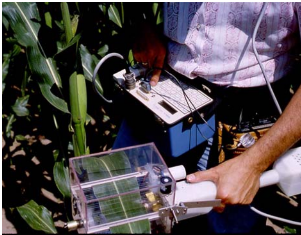
Figure 8: The first prototype of LI-COR's implementation of John's photosynthesis system had the IRGA in the handle.
