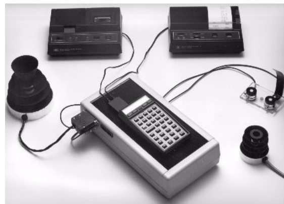
Figure 14: The product that never was. A data logger, based on HP-IL interface, with two Pine Cone Sensors (large and small) attached.
