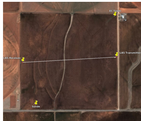
Figure 1. Experimental setup at FC01 showing EC tower (NE corner), Sonde location (SW corner) and the LAS path (middle of field).
