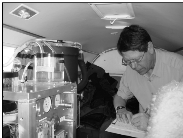
Figure 3. The author is shown aft in N234K, noting the condition of various AINC systems. A forepump attached to the sampling inlet was used to ensure adequate sampling of air external to the pressurized cabin.
