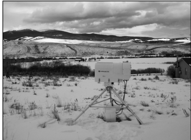
Figure 2. The WMI Radiometrics WVR-1100 dual-channel radiometer at Cedar Creek, shown sampling at the 110° azimuth. Kennaday Peak, Medicine Bow Range, is visible in the upper left.
