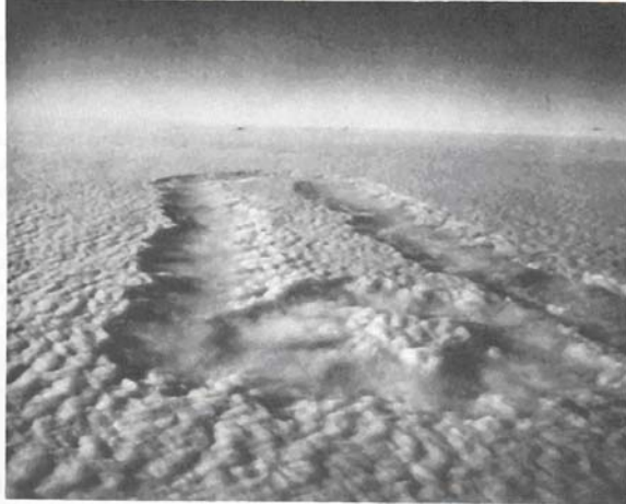
Figure 3. Racetrack pattern approximately 20 miles long produced by dropping crushed dry ice from an airplane. The safety pin-like loop at the near end of the pattern resulted when the dry ice dispenser was inadvertently left running as the airplane began climbing to attain altitude from which to photograph results. [From Havens et al. (1978). Photo courtesy of Dr. Vincent Schaefer.]
