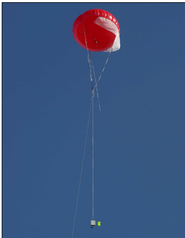
Figure 1. SkyDoc aerostat balloon carrying the aerosol instrumentation.
