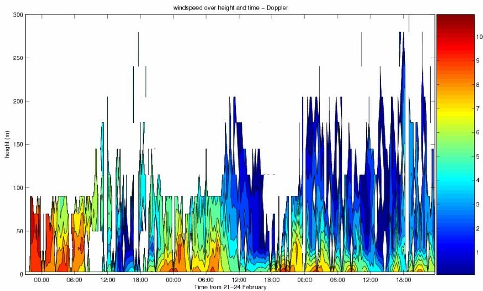
Figure 3 Wind speed over height and time from the Doppler Sodar (15 minute averages every 15 minutes), for 21-24 February 2002. The lowest level is provided by the AWS at the same location. Note that the AWS observations are taken at a height of 3 m, while the lowest Doppler level is at 30 m. This causes the gradients in the lowest levels.
