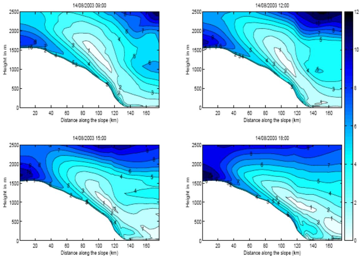
Figure 1 A vertical cross-section showing wind speeds along the slope near Halley Research Station, for the 14<sup>th</sup> of August 09:00, 12:00, 15:00 and 18:00.
