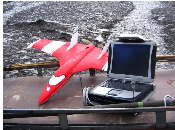
Figure 1: SUMO airframe based on the model construction kit FunJet by Multiplex and the Panasonic CF-19 Toughbook used as ground control station.
