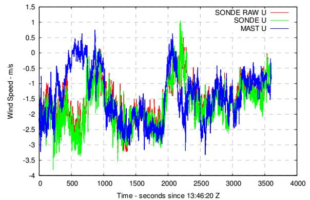
Figure 4. Time series of wind speed (u) collected from the sonde without motion correction (red), with motion correction (green) and data collected from a nearby mast at the same height (blue)
