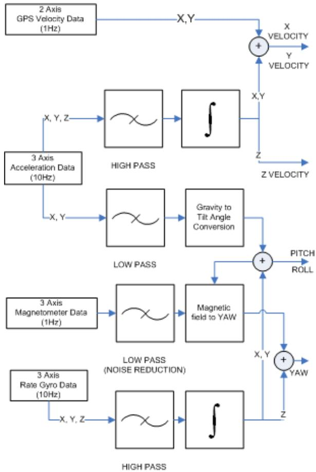
Figure 3. Block diagram of the motion correction algorithm
