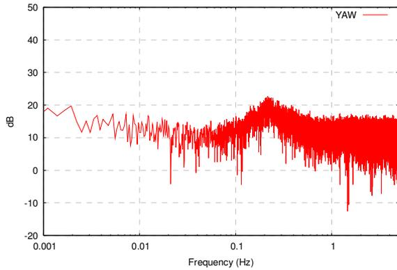
**Figure 6.** Power spectrum of sonde Yaw motion.
