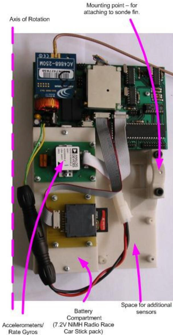
**Figure 2.** Internal instrument electronics and mountings. System extracted from body for clarity.
