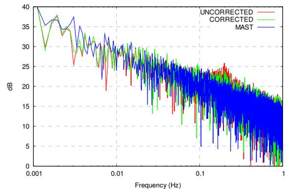
Figure 5. Power spectrum of sonde uncorrected (red), corrected (green) and mast wind speeds
