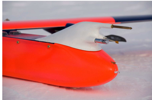
Fig. 1: The measurement nose with the 5HP, Vaisala Intericap and Dantec foil temperature sensor mounted.
