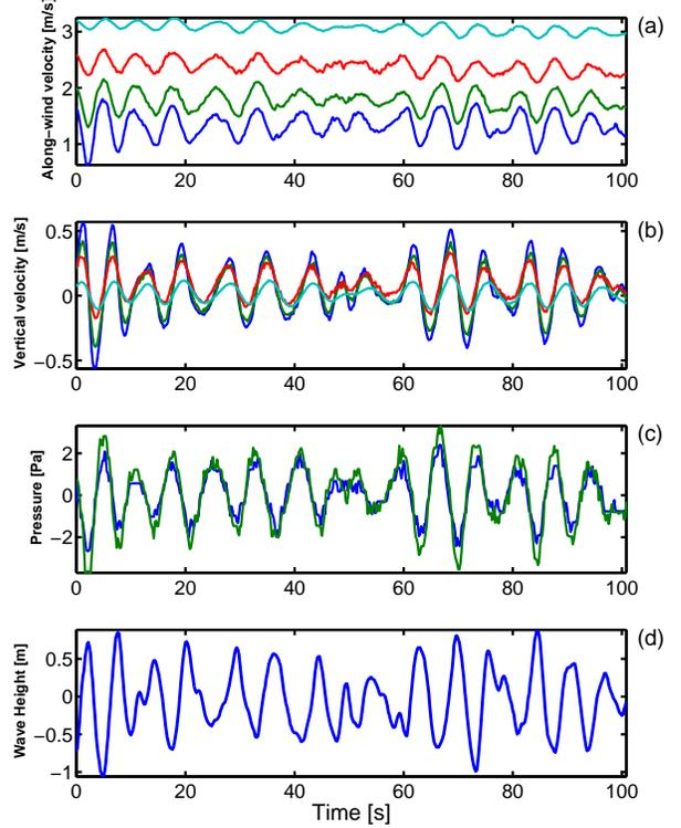
Figure 2: A low-wind regime frequently observed during CBLAST. Time-series over 100s of (a) horizontal along-wind velocity, (b) vertical velocity, (c) pressure, and (d) surface elevation. The colors in the velocity plots correspond to instruments heights, in the order blue (the lowest), green, red and cyan (the highest).
