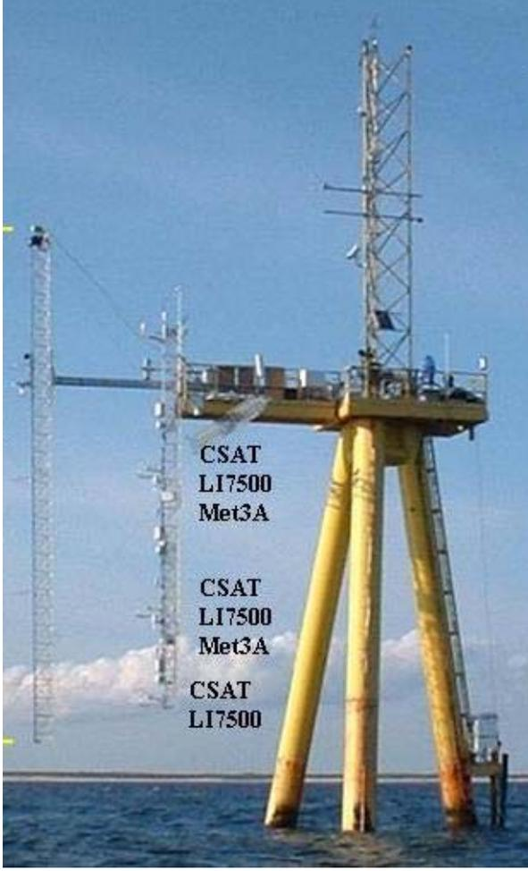
Figure 1: Air-Sea Interaction Tower during the Coupled Boundary Layers Air-Sea Transfer (CBLAST) experiment with the instruments mast. A photograph by Dr. J. Edson.
