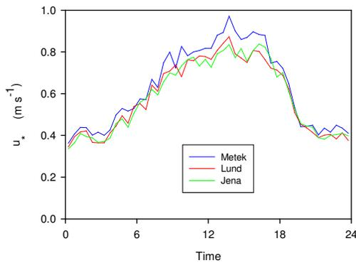
Figure 3. Average diurnal variation of friction velocity, June 7-9 and 11-13, 2008
