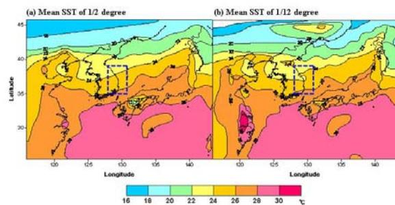
Fig. 3. Mean SST distribution of (a) 1/2 and (b) 1/12 degree grid used during modeling period.
