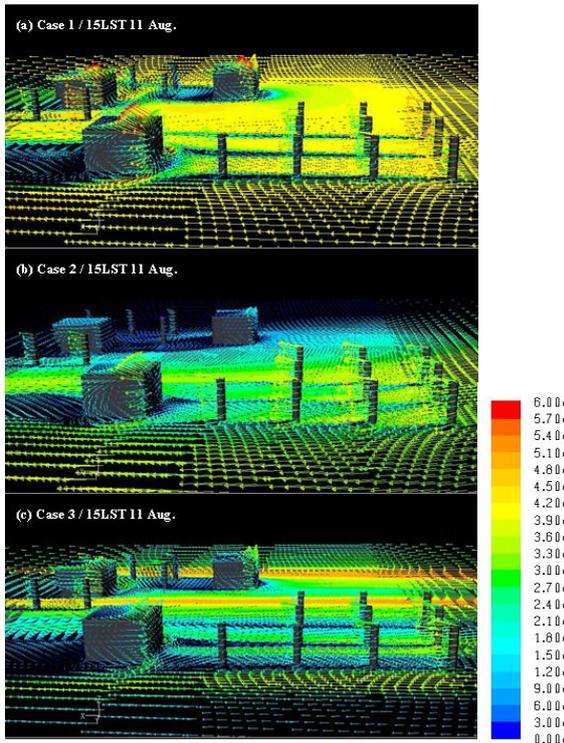
Fig. 6. Wind vectors ( $\text{m s}^{-1}$ ) simulated with FLUENT in the idealized city block at 1500 LST 11 August 2007.
