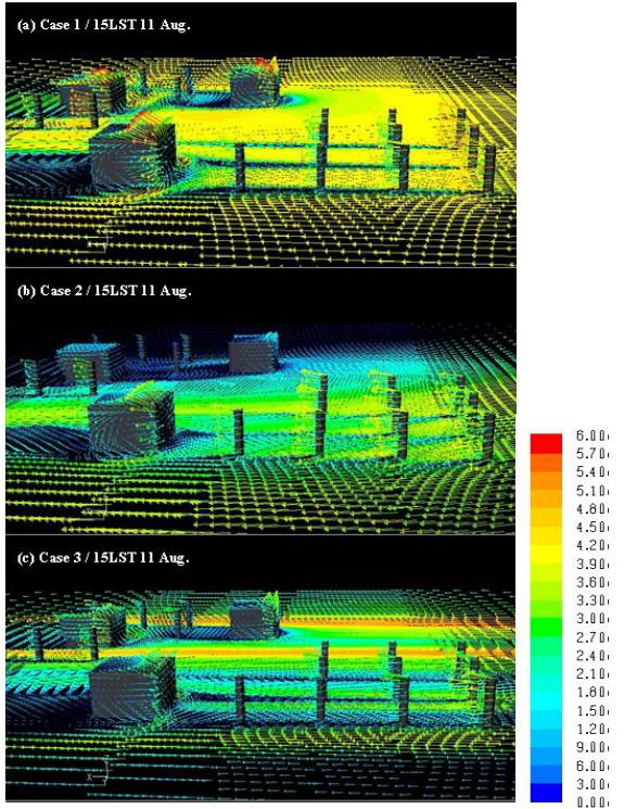
Fig. 6. Wind vectors ( $\text{m s}^{-1}$ ) simulated with FLUENT in the idealized city block at 1500 LST 11 August 2007.
