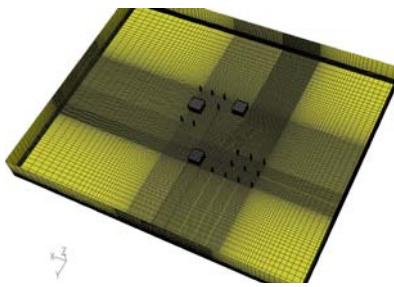
Fig. 2. The computational domain for the FLUENT simulations depicted as an idealized city block.
