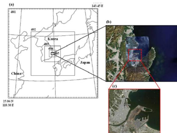
Fig. 1. Modeling domains. (a) Five nested grids with horizontal grid resolutions of 40.5 (d01), 13.5 (d02), 4.5 (d03), 1.5 (d04) and 0.5 (d05) km used in WRF model. Domain is enlarged from the left to the upper right and the lower right. (b) Topographic details of last domain (d05) and (c) domain for FLUENT modeling.
