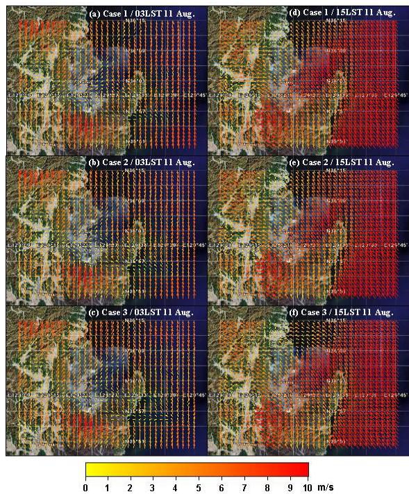
Fig. 4. Wind fields at 10 m above ground level simulated with WRF on the fine grid (d05). (a) case 1, (b) case 2 and (c) case 3 at 0300 LST and (d) case 1, (e) case 2 and (f) case 3 at 1500 LST 11 August 2007.
