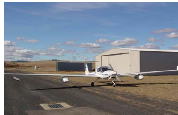
Figure 3: ECO-Dimona instrumented motorized glider operated by Airborne Research Australia
