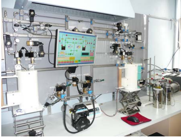
Figure 2: Laboratory apparatus for extraction of radon from airborne sampler charcoal traps and delivery to Lucas cells for counting
