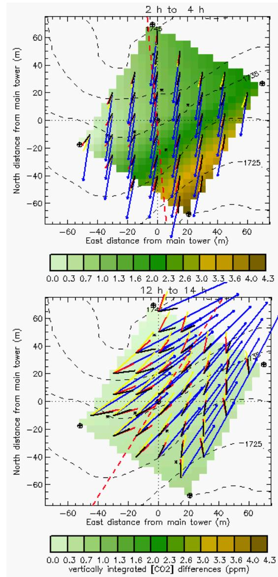
Fig. 2: Flow patterns and CO<sub>2</sub> concentration distribution (vertically integrated at gridpoints) in the control volume for local conditions during nighttime (top) and daytime (bottom). Black, red, yellow and blue arrows refer to wind vectors at levels 1.5, 6, 12 and 30 m a.g.l., respectively. A wind speed of 1 m s<sup>-1</sup> is scaled with 25 m on  $xy$ -axis.
