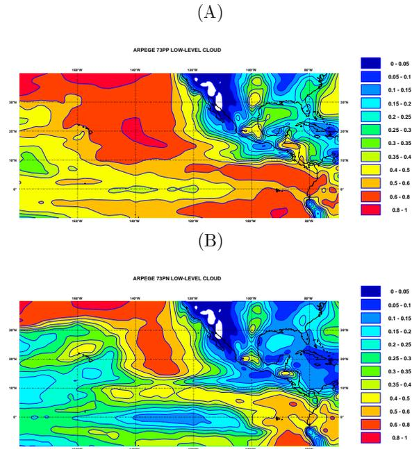
Figure 3: A: low-level clouds from ARPEGE with TKE+KFB (June 2007). B : low-level clouds from ARPEGE with TKE+KFB + thermal production from KFB + modified mixing length (June 2007)
