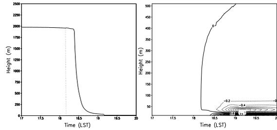
Fig. 2. Temporal evolution of the (a) PBL height from the new (solid) and old (dotted) SBL schemes and (b) the vertical profiles of the differences in potential temperature (new minus old).
